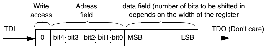
Figure 48-7. TDI/TDO on write access
